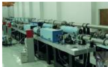
(b) The ninth beam of SG-II facility, which was built in 2005 as a probe and high-pressure shock-wave driver; its output reaches 5.2 kJ per pulse with a beam aperture of 350 mm.
