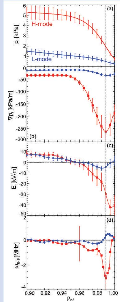
Fig. 1: (a) Main ion pressure and its gradient (b), (c) radial electric field and (d)  $E \times B$  velocity shear.
