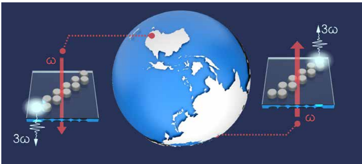
Concept of nonlinear parametric topological edge states as seen from Canberra and from Moscow perspective. Third-harmonic generation from edge states in a zigzag array of silicon nanoresonators depends on the pump direction.
