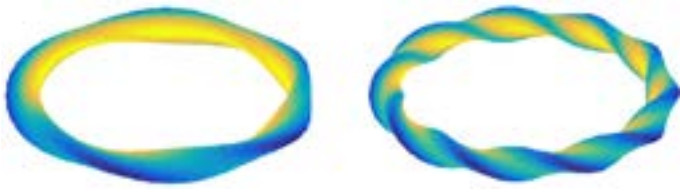
Figure 1. A magnetic surface in a classical stellarator with N_p = 5 (left) and N_p = 10 (right). Colour indicates the amplitude of B on the surface. [7]
